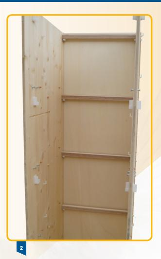
Then, from the top to the bottom, push the rear crossbars with the dimensions 19 x 27 mm onto the metal bolts on the side panels. 5 bars in total.
