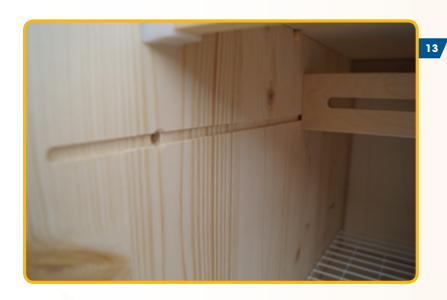
In doing so, the dowel on the front face is guided in the groove on the side panel until it meets and engages
