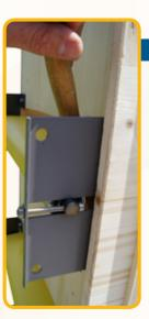
Then fit the second bearing plate on the front and secure it with two hexagonal nuts. Then push the shaft forward again with a hammer handle and unscrew the hexagonal nuts on the tensioning screw.
