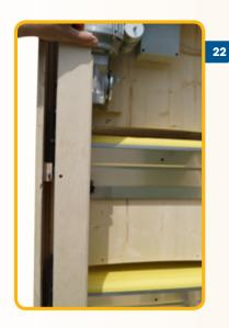
Refit the chain guard and securely tighten the 6 mm nut with washer with
