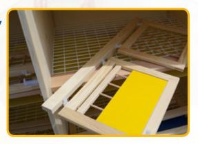
Then from the outside fit the front doors onto the hooks.
