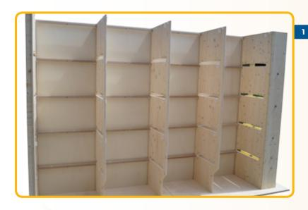
If the box is delivered with a rear panel, insert the panel in the grooves at the back of the side panels. Then, from the top to the bottom, push the rear crossbars with the dimensions 19 x 27 mm onto the metal bolts on the side panels. 5 bars in total. In doing
