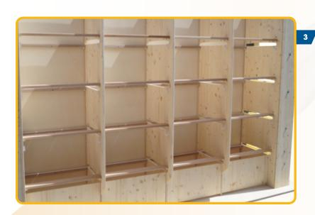
Press the beech wood perch bars onto the metal bolts on the upright side panels. 4 pieces per section. In doing so the notch on the bars must always point to the back. Important: With the box sizes 69.2 cm, 59.2 cm and 54.2 cm, the bars are marked with the numbers 1 and 2. The bars with the number 1 are fitted in the top row of the section. The bars with the number 2 in the second row from the top, and so on.
