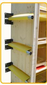
Feed the return shaft complete with the screwed-in screws through the droppings belt up to and into the rear bearing plate. Important: The connecting joints of the shafts must always point outwards.
