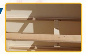
Press the beech wood perch bars onto the metal bolts on the upright side walls. 4 pieces per section. In doing so the notch on the bars must always point to the back.
