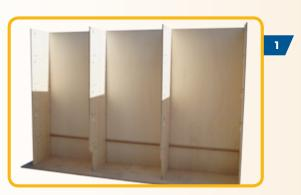
If the box is delivered with a rear panel, insert the panel in the grooves at the back of the side panels. Then, from the top to the bottom, push the rear crossbars with the dimensions 19 x 27 mm onto the metal bolts on the side walls. 5 bars in total. In doing so, the holes in the rear crossbars must always be facing forward.
