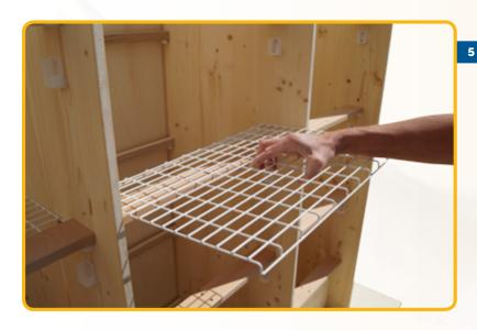
Now the wire meshes are inserted. The folds must point downwards.
