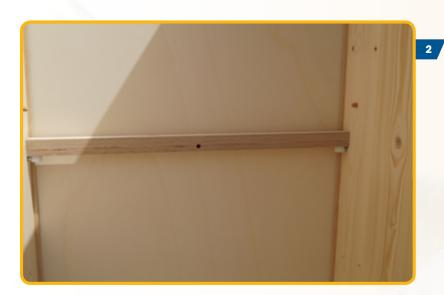
In doing so, the holes in the rear bars must always point to the front.
