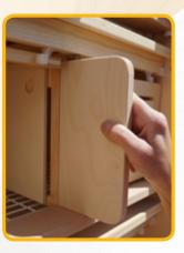
Fit the dividing piece. The dowel with the metal spring is inserted into the hole of the cross bar and pressed up. Now carefully move the dividing piece to the side until it snaps into the two holes of the perch bar.
