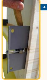
Then fit the second bearing plate on the front and secure it with two hexagonal nuts. Then push the shaft forward again with a hammer handle and unscrew the hexagonal nuts on the tensioning screw.
