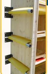
Feed the return shaft complete with the screwed-in screws through the droppings belt up to and into the rear bearing plate. Important: The connecting joints of the shafts must always point outwards.
