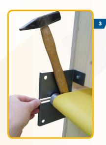
Unscrew the hexagonal nut. Tip: The shaft can easily be levered slightly forward using a hammer handle.
