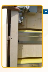
Refit the chain guard and securely tighten the 6 mm nut with washer with a socket wrench.
