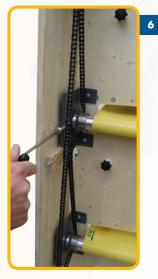
Remove the chain guard on the drive side.
