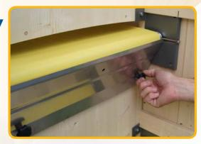
Fit the scraper blade and firmly screw it on.
